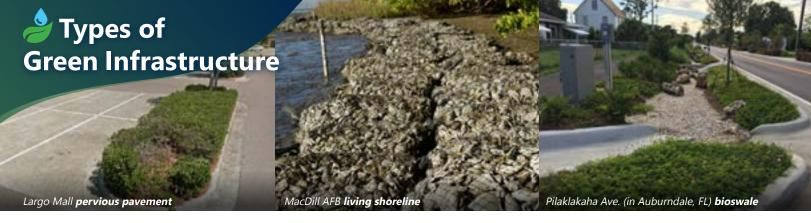
Bioswale: A ditch or swale that has been modified and planted with Florida-Friendly vegetation to increase pollutant removal and water infiltration.
