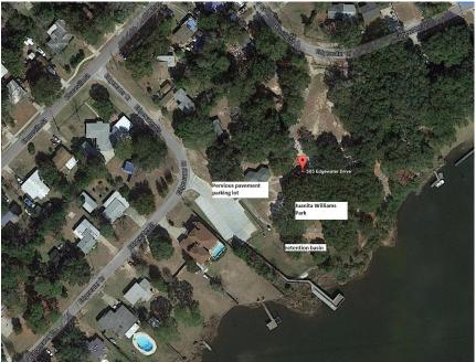
The project was undertaken to remove and replace an existing 8,770-sf gravel/dirt parking lot. Since Bayou Chico is an impaired water body, the County needed to ensure that the postdevelopment nutrient loading was less than the pre-development nutrient loading. Additionally, the County wanted to demonstrate the use of pervious pavement as an LID BMP
