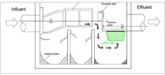
Figure 5.13.1a. Off-line Up-Flow Filter Schematic
