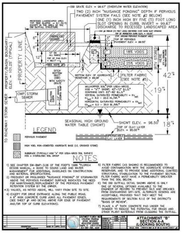
Figure 5.9.9. Pervious Pavement Site Plan
