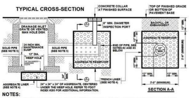
Figure 5.4.2. Typical Exfiltration Trench Sumps and Dead End Details
