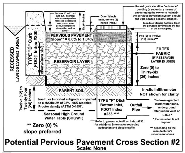
Figure 5.9.3. Pervious Pavement System Cross Section #2
