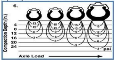
Up to 80% of compaction occurs during the first pass of a vehicle!
