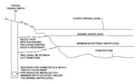
Figure 5.12.2. Schematic for a Typical Stormwater Harvesting Pond
