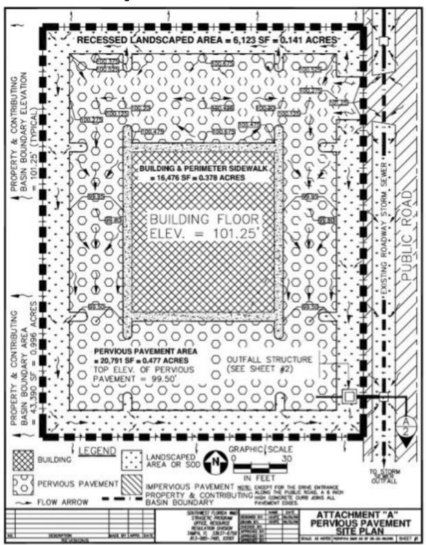
Figure 5.9.8. Pervious Pavement Site Plan
