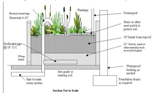
Figure 5.15.4. Example Stormwater Planter Box Biofiltration System
