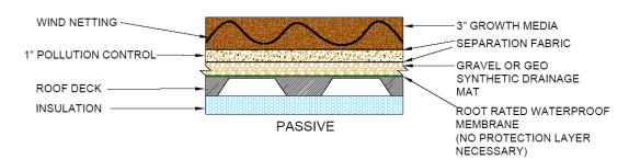
Figure 5.10.1a. Extensive Greenroof Section (Usually Passive Function)
