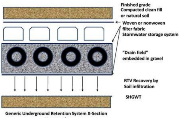
Figure 5.5.1. Generic Underground Retention System
