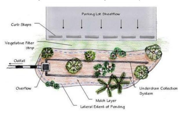
Figure 5.15.1. Plan View Illustrating a Biofiltration System
