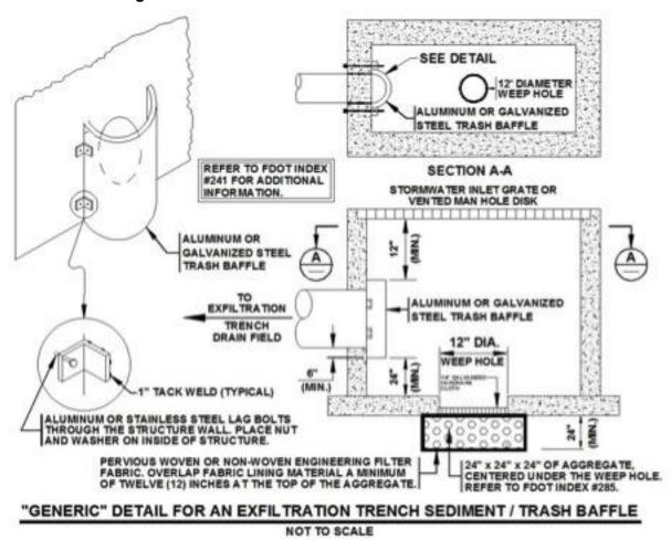
Figure 5.4.3. Detail for Exfiltration Trench Trash Baffle
