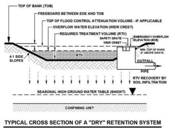
Figure 5.3.1. Typical Cross-section of "Dry" Retention Basin
