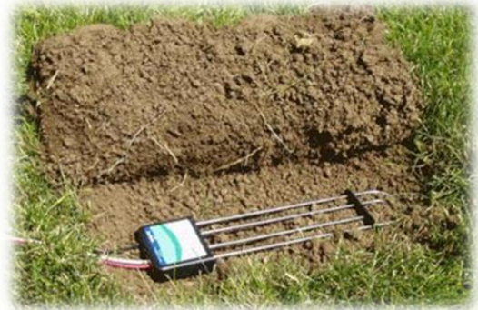
A soil moisture sensor, buried in the turf root zone prevents irrigation when it is not needed.
